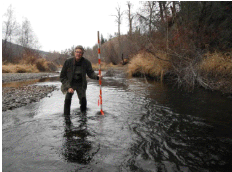
Photo 3 Looking upstream from proposed weir location to illustrate expected relative increase in residual pool depth after weir installation (upper orange flag)
