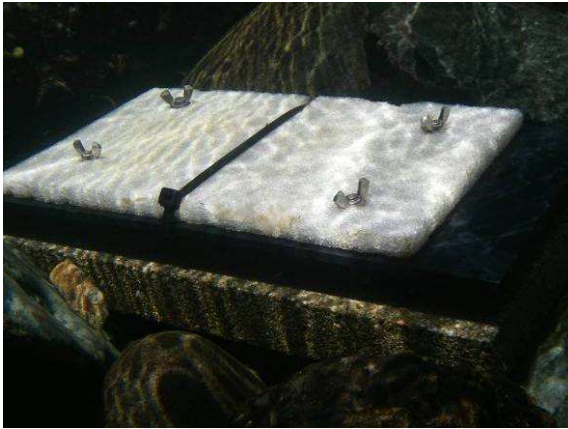
Figure 2. Periphyton collector plate secured to stream bed with cobbles.
